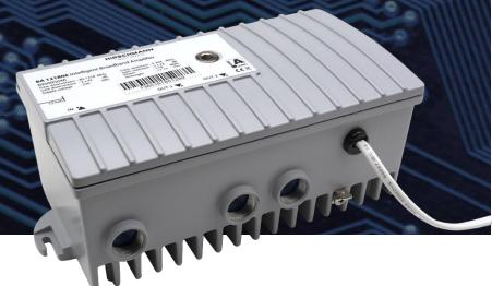
The modular design offers multiple bandwidth options within its 85 - 1218 MHz downstream and 5 - 204 MHz upstream range. With the option to easily replace the diplex filters, depending on the required bandwidth. All adjustments and settings are realized by the built-in microprocessor. These settings can be changed via a smartphone or tablet through a separate Bluetooth dongle.
